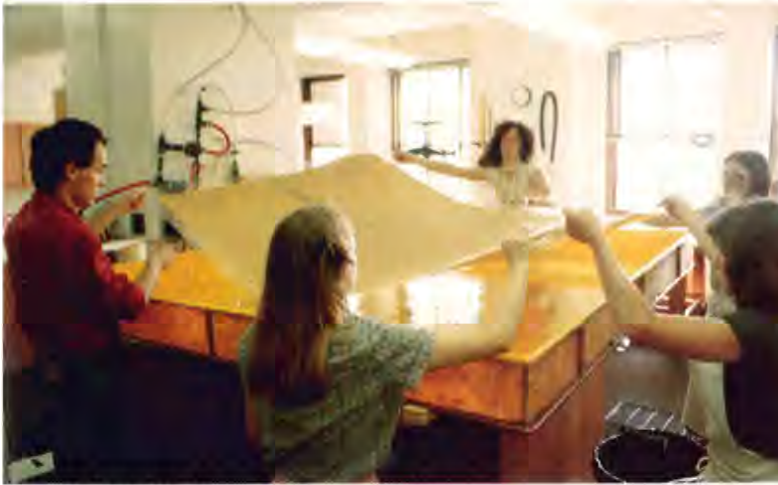
At Philadelphia's Conservation Center for Art and Historic Artifacts, "Mylar" is employed in removal of deteriorated backings from old maps and other artifacts.
