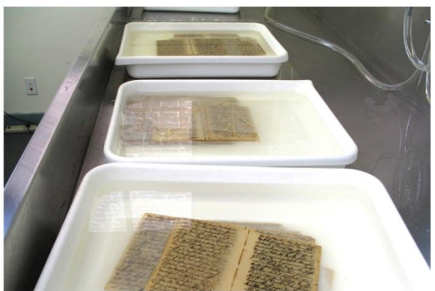
FIG. 6. The yellow water in the far tray indicates the need for more washing; the leaves in the near tray are clean.
