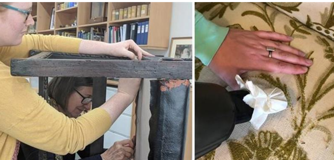
(Left) exit holes from past pest damage; (Right) careful vacuuming of upholstery using a covered nozzle; Images courtesy of Jess Chloros and Rachel Bissonette
