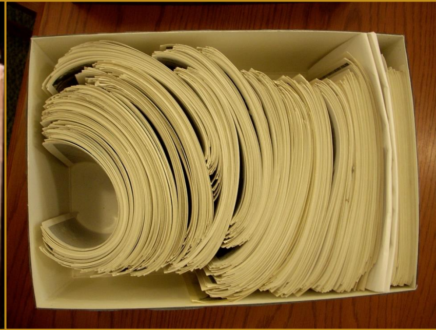
Improper Vertical Storage
